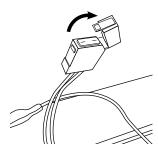
**3** Open the fuse cover to expose the fuse
